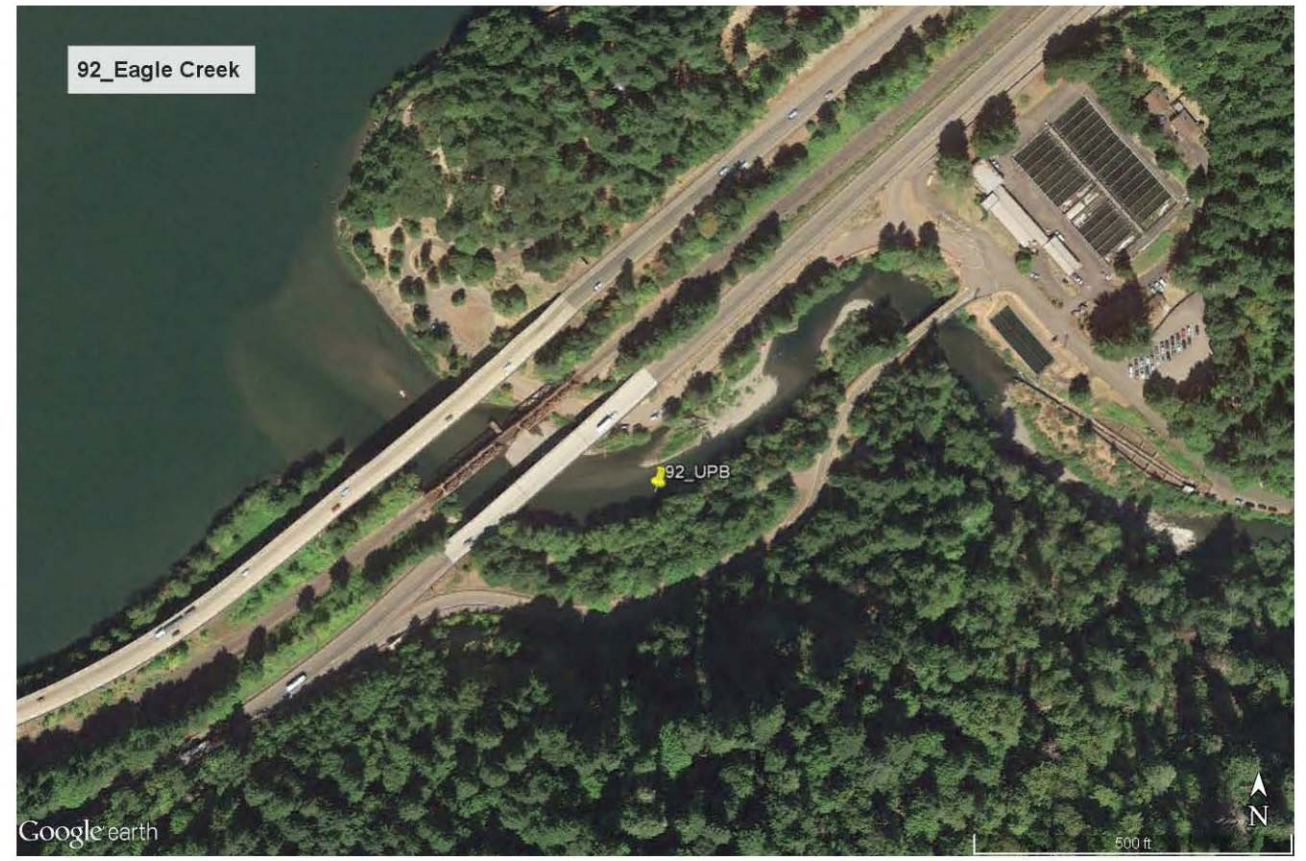
The upstream extent was set at a riffle 0.15 miles (0.24 km) upstream that constrains movement (depth of 0.8 meter or less), based on a site visit conducted on 8/17/17.
